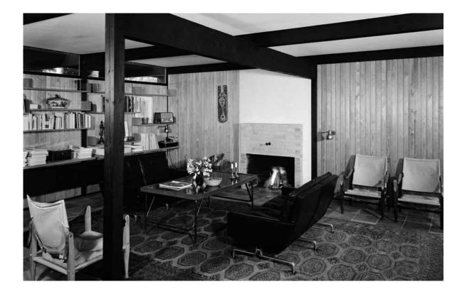
The most distinctive room in the house is the living room with a square floorplan 6.7 m across and three bays measuring 2.1 m along the length of the house and grey slate flooring with 30 x 30 cm tiles and bricked fireplace on the floor. The three large windows to the south light up the room and bind it with the garden outside.
